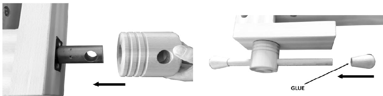
**Hint.:** Smear inside knob as well as wrench by glue and put together. Wipe off excess glue with a cloth. **Wait at least 1 hour before using.** Repeat the same on the front vice.
